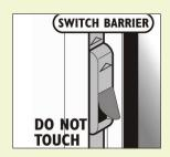
The switch barrier projecting from the locking mechanism, adjacent to the handle, is a safety device. It ensures that only one mode ('tilt' or 'turn') can be selected at any one time, by securing the handle into the selected mode, while the window is open.
